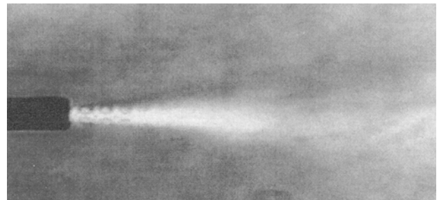
Fig. 6 Schlieren image of jet blasting nozzle below design pressure
